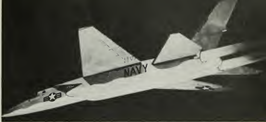
DUAL PIPES—Artist's painting shows Navy's new carrier-based A3J-1 now being tested. It will provide the Fleet with a supersonic weapons system.
